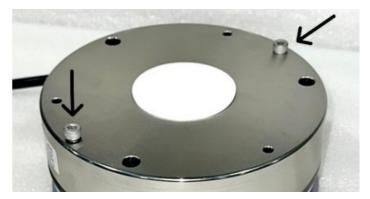
To disengage the **EMB**, locate the two 4 mm Allen head screws on the motor. These screws sit finger-tight at rest. To release the parking brake, tighten both screws, which pulls the plate away from the motor. Always keep a 4 mm Allen key handy for this procedure.
