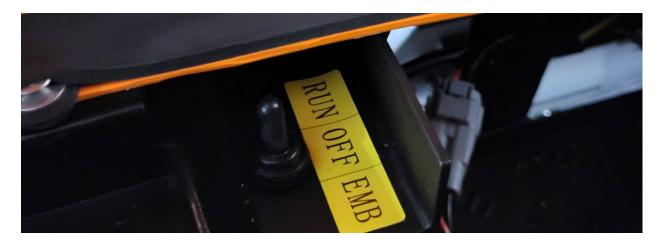
The **RUN/OFF/EMB** switch is located under the seat where the battery compartment. Before using the car, ensure the switch is in the "**Run**" position. When storing or working on the unit place the cart in OFF position. When towing or pushing the cart, toggle to "**EMB**" position. "**EMB**" releases the emergency brake, allowing the cart to move. **Please note:** The cart's battery must have power for the **EMB** feature to work properly.
